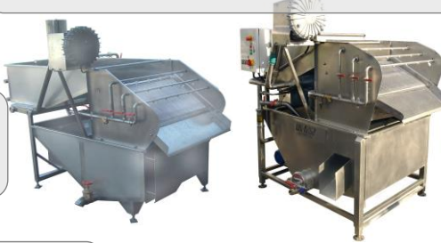
WASHERS – Used for initial washing with air support. Initial washing in water closed circle, final cleaning with fresh water sprinklers. Unit is equipped with pump, slotted sieve and air turbine.
