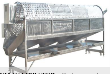
DRUM CALIBRATOR – Used to separating product on fractions, calibrating champignons using sieve with round shaped holes. Sieve shape and hole size are set depending on processed product and client needs.
