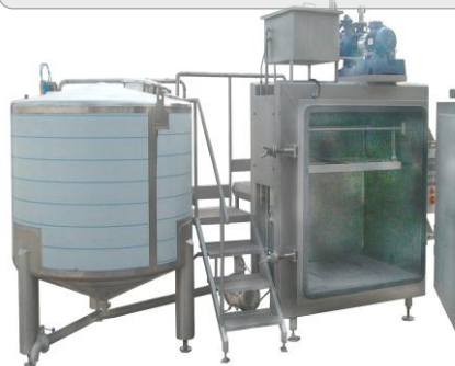
VACUUM CHAMBER – Used to structural saturate mushrooms with water or solution. Level can be regulated up to 60%. Capacity (3-4) cycles/h.
